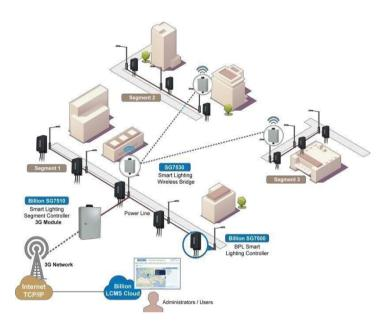
Fig.2 Data flow diagram for smart street lights.
